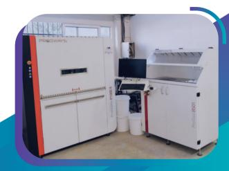
The machine has a production volume of 300 x 300 x 300 mm<sup>3</sup>.
